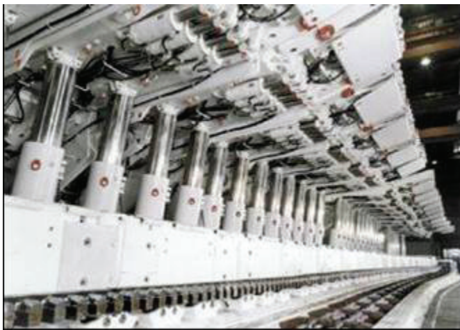
Roof Supports (Shields) for Longwall Mining
