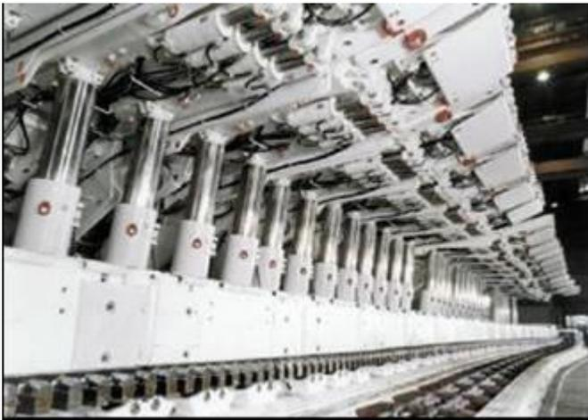
Roof Supports (Shields) for Longwall Mining
